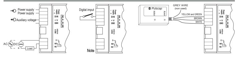
Note: The absence of power supply also causes the lack of auxiliary voltage and then in addition to the blackout alarm, the opening of the contact at the input will also be signaled.
